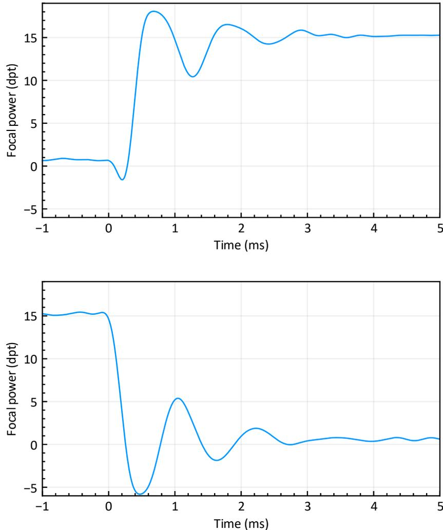
Figure 10: 80% step response of the EL-3-10 lens
