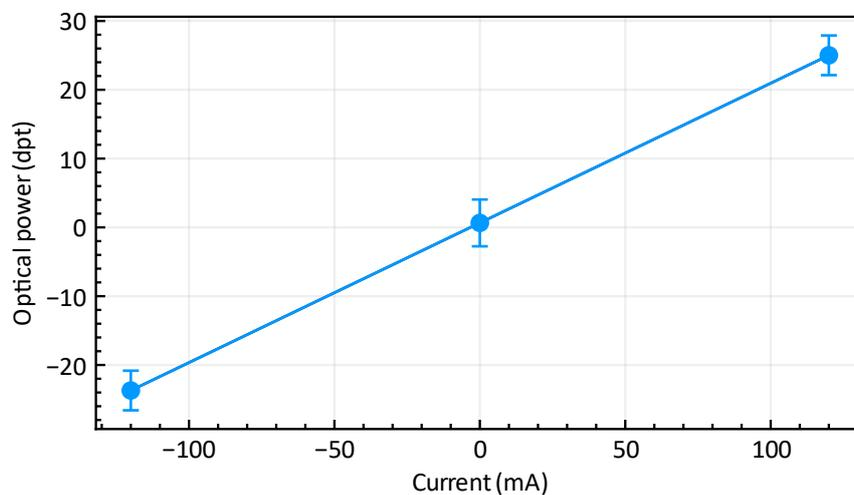
Figure 7: EL-3-10 typical current vs optical power graph
