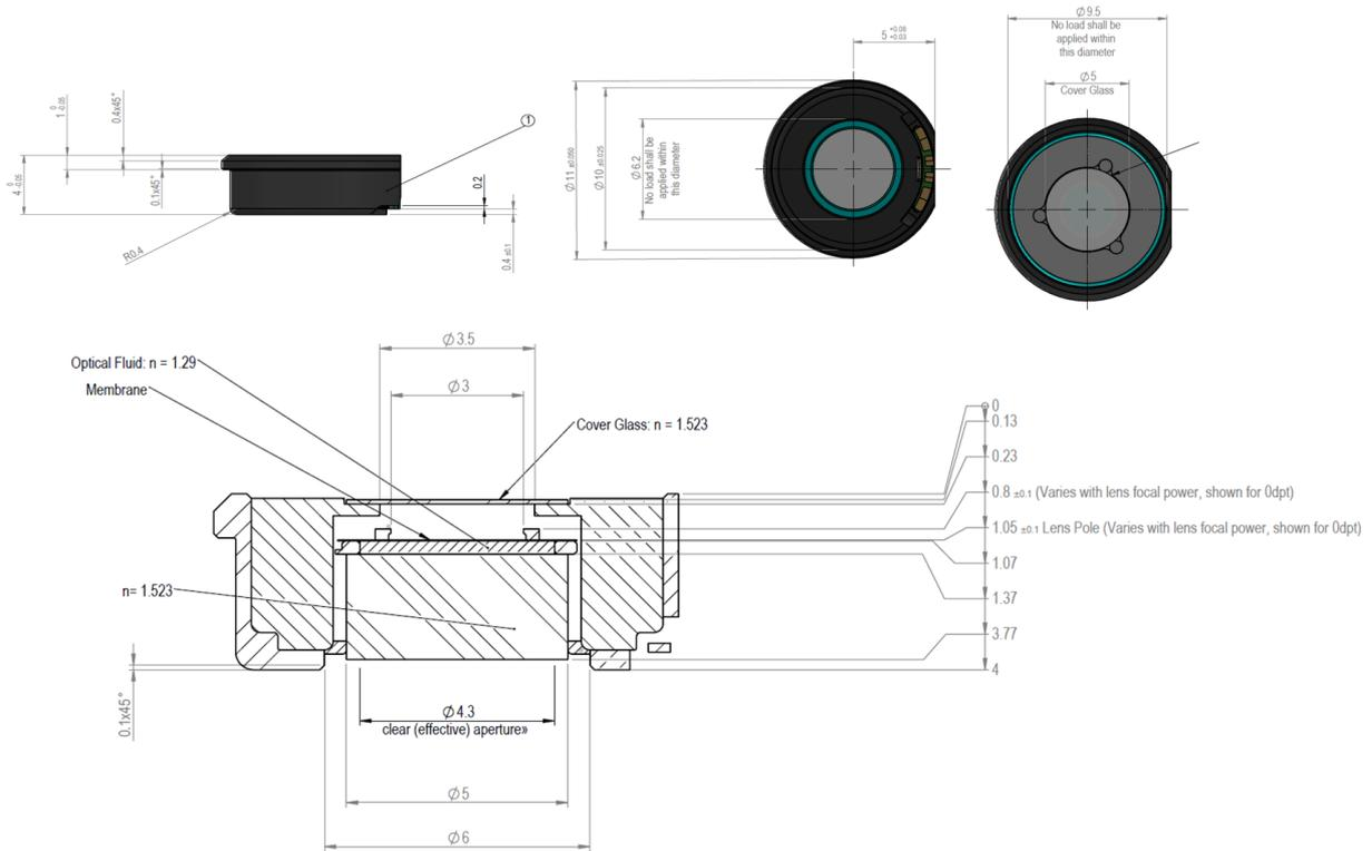
Figure 1: Mechanical drawing of the EL-3-10-XXX-26D-OEM lens
