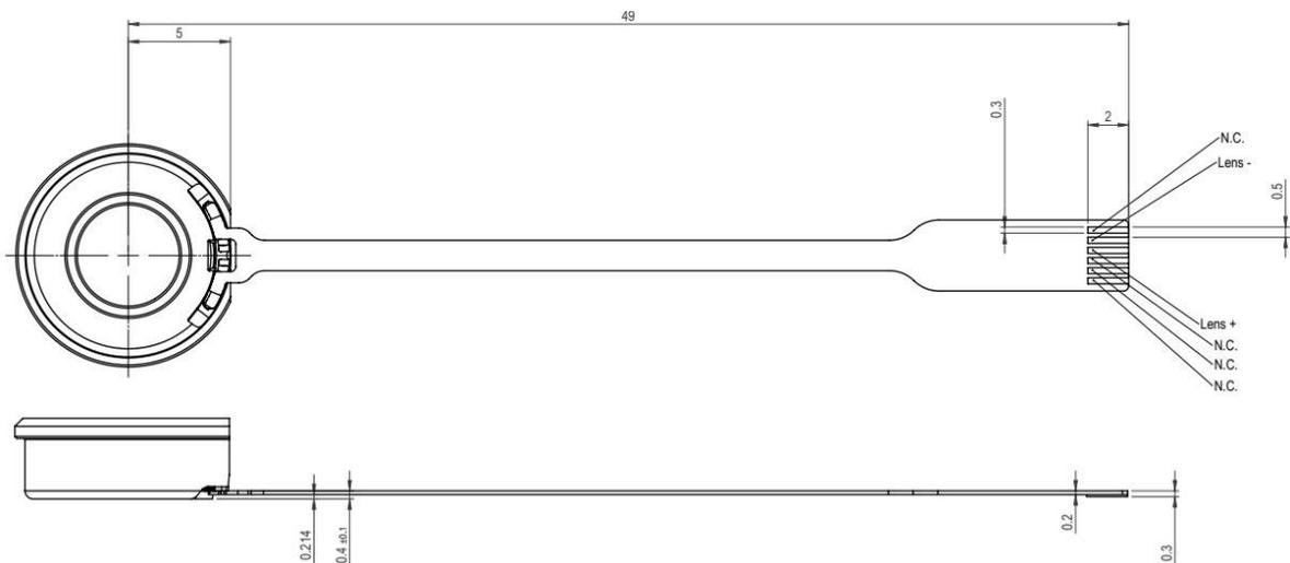
Figure 2: Mechanical drawing of the EL-3-10-XXX-26D-FPC lens
